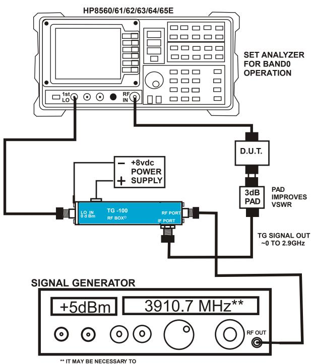
\*\* IT MAY BE NECESSARY TO TUNE IN THE FREQUENCY. TUNE FOR MAXIMUM AMPLITUDE WITH THRUOGH AS DUT
